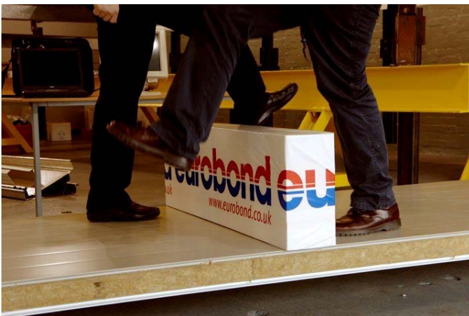
EB500 test. Two men cross over 450mm high step at mid span
