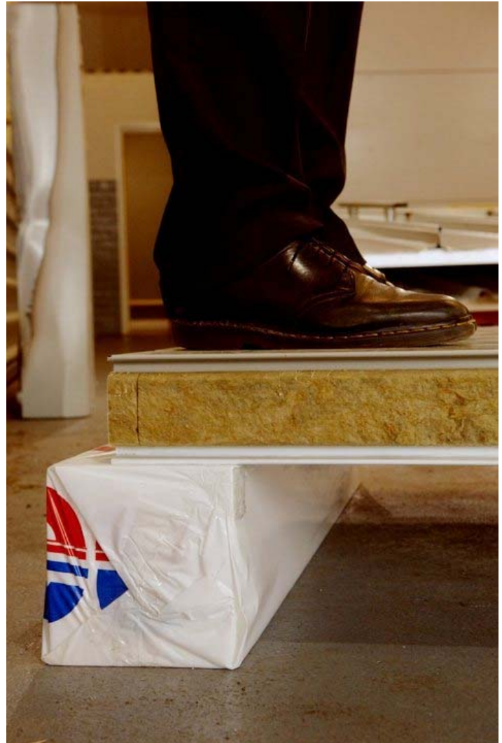
EB500 test. Panel is simply supported over 6m span
